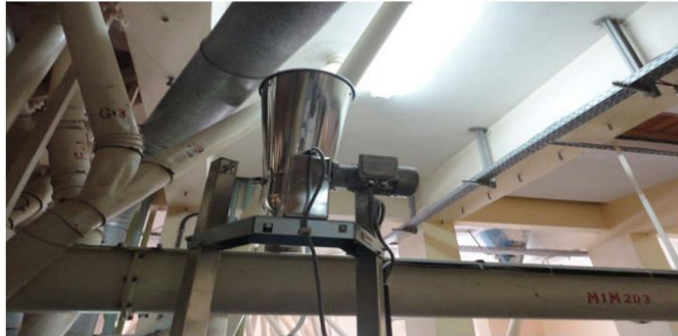
Micro-feeder fitted above mixing conveyer.
