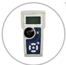
iCheck Iron measures absorption of 525 nm by the red complex.
