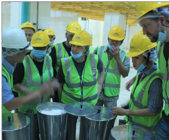
EMT members and observers toured a flour mill in Viet Nam in April 2018. The open container is a feeder with vitamin and minerals to be added to flour. Photo by Bob Lubitz.
