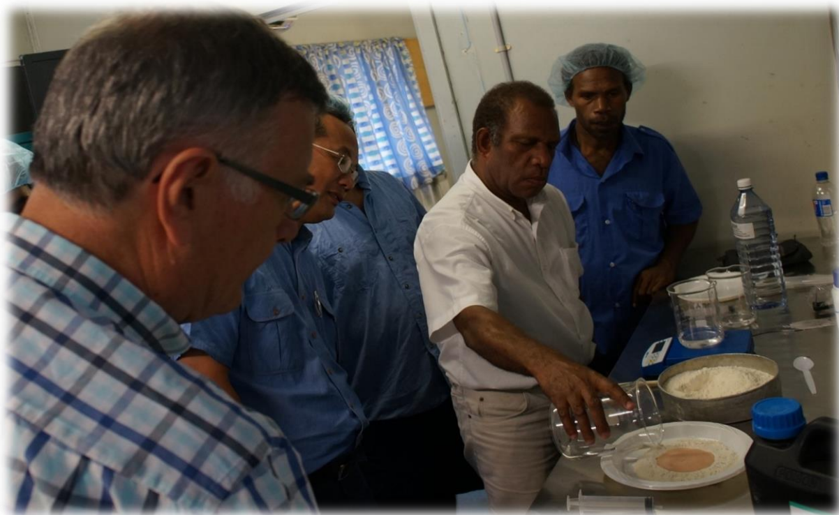
Quentin Johnson, left, our Training and Technical Support Coordinator, observes as newly trained flour millers in Solomon Islands perform the iron spot test, a qualitative method to indicate whether flour has been fortified. Photo by Becky Tsang.
