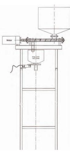
Figure A5. Screw feeder system
