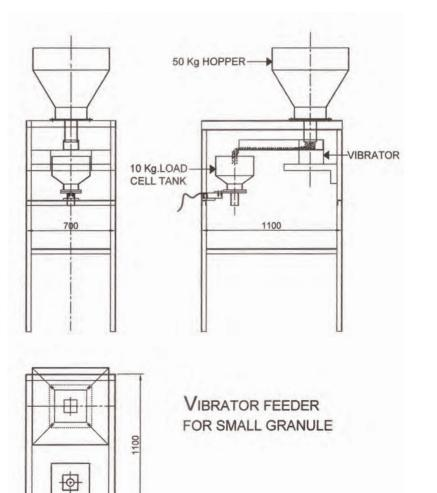
Figure A4. Vibrator feeder
