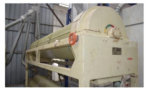
**Figure A11**. Example blending setup – rice length grader adapted for use as a horizontal blender
