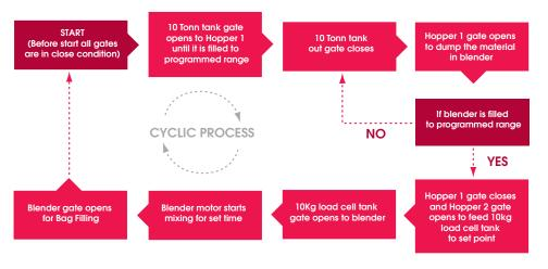
Figure A1. Logic of the PLC program
