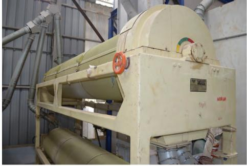
Figure 5.4. Rice length grader adapted for use as a continuous horizontal blender
