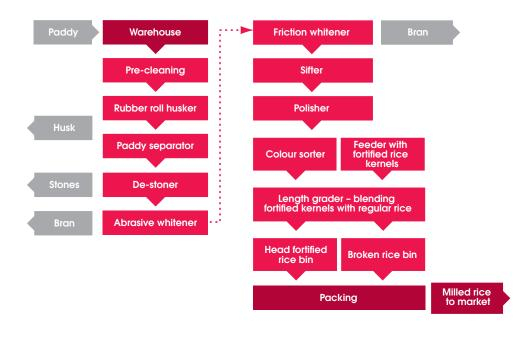
**Figure 3.5.** Typical flow chart of fortified rice mill – transforming length grader into blender
