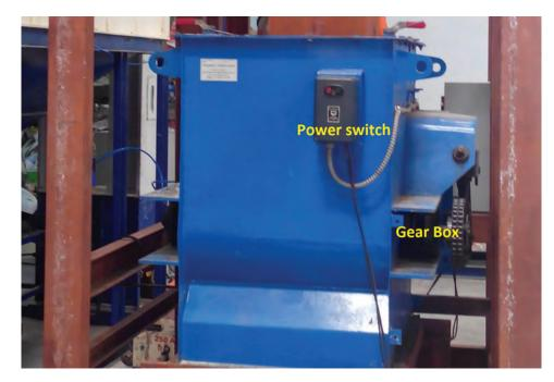
Figure 5.3. Side view of the Forberg fluidised bed blender
