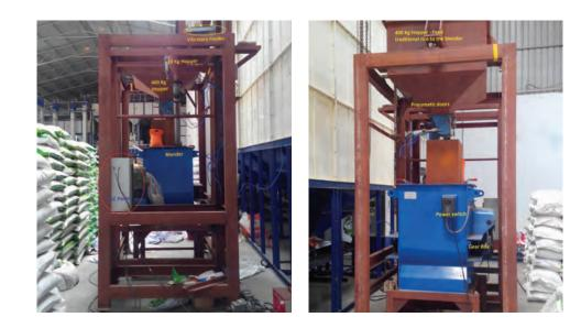
Figure 3.1. Framework for integration of vibratory feeder with Forberg blender
