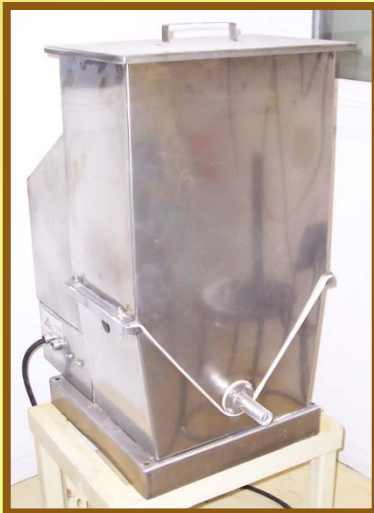
Type one类型1: Screw Feeder螺旋喂料
