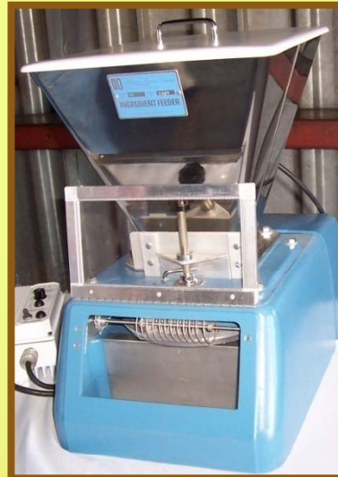
Type two类型2: Revolving Disk旋转盘
