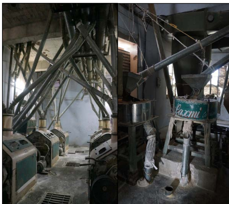
Figure 12: Roller flourmill (L), chakki mill integrated with roller flourmill (R)
