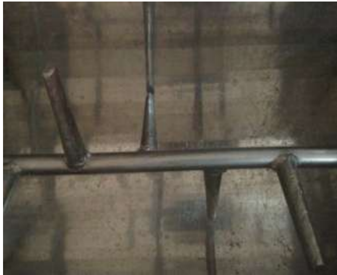
Figure 25. Pin-type blades for wet flour mixing
