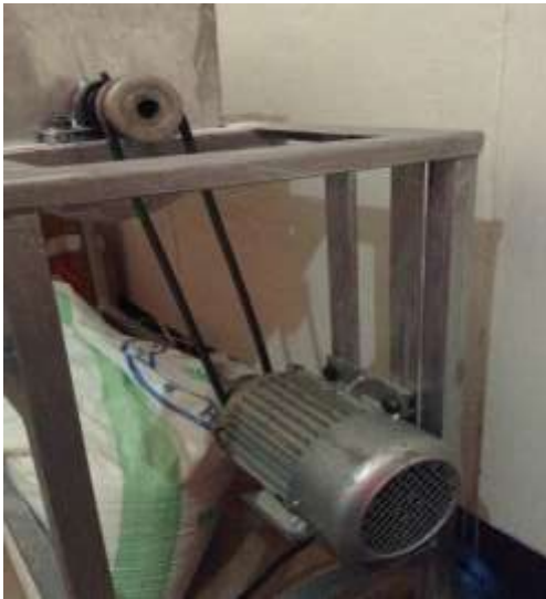
Figure 24. Power transmission for horizontal mixer
