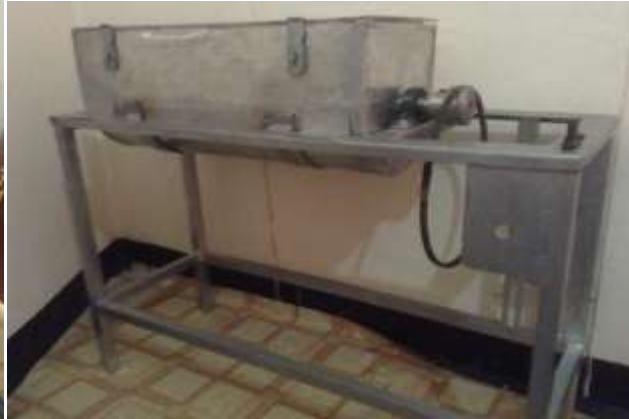
Figure 23. As-built horizontal agitator
